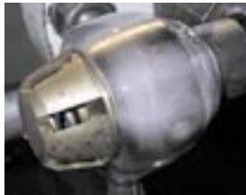
TDA test performed by the Swedish Navy at a temperature of 1°, a flowrate of 75l/min and 70 meters of depth
